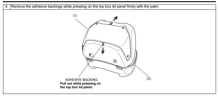
5. Applying adequate pressure of 5 kgf (50 N) to the attached top box lid panel, and then release the adequate pressure and leave the top box lid panel for 10 minutes to stabilize the fitting of the adhesive surface.
